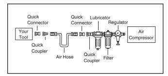
**Figure 2.** Installing your tool.
